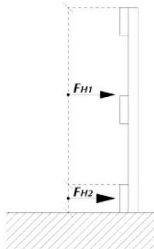
**Figure 8 — Charge limite ultime, alternative 1**
